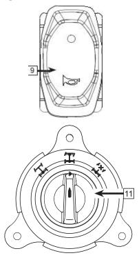
On-Command 2WD / 4WD / 4WD-LOCK Switch Operation
