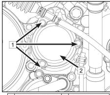
1. Use a new drain bolt washer and tighten it to specified torque.
