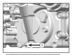
1 Drain bolt, Transmission
