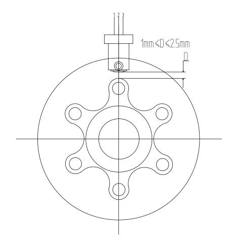
Note: Always screw in the sensor by hand when installation or adjustment.
