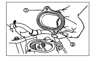
2.Inspect: •Electrode ① Wear/ damage --> Replace. ●Insulator ② Abnormal color → Replace. Normal color is a medium - to- light tan color. 3.Clean: Spark plug (with spark plug cleaner or wire brush) 4.Measure: •Spark plug gap ③ (with a wire gauge) Out of specification  $\rightarrow$  Adjust gap.
