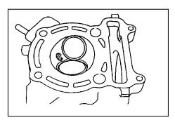
●Cylinder head Scratches/damage → Replace.
