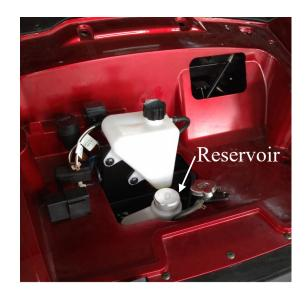
7. Hold brake pedal on to maintain pedal pressure, and open bleeder screw. Close bleeder screw and release foot pedal.
