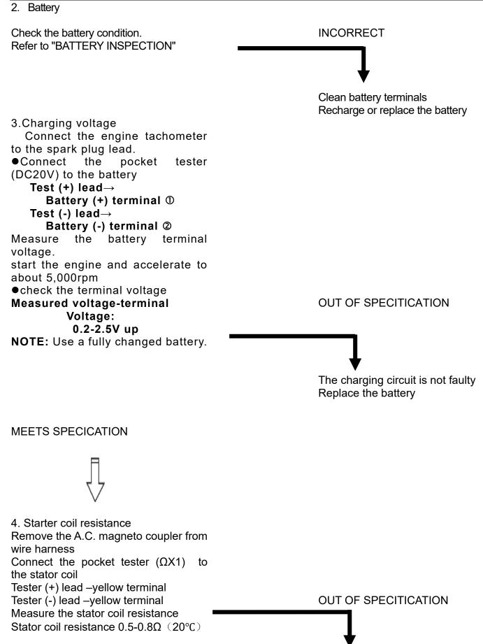
Replace the stator coil
