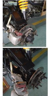
5. Loosen two bolts that secure the rear knuckle to the A-arm. Remove the rear knuckle assembly by sliding it off of the axle.
