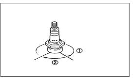
Before removing the spark plug, use compressed air to blow away any dirt accumulated in the spark plug well to prevent it from falling into the cylinder.
