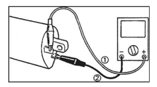
Tester (+) lead Spark plug lead Tester (— ) lead Pink Terminal
