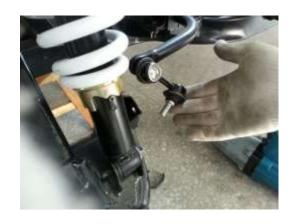
4. Remove the two bolts that secure the stabilizer bar to the main frame, each side.
