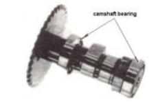
9. Check camshaft bearing for looseness and wear and tear and sprocket for abnormal wear. If so, replace as a whole.
