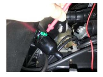
Check the pickup coil has the specified resistance.
