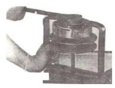
17. Remove clutch locknut.
