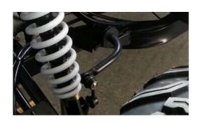
8. Reverse the procedure for installation. Torque the stabilizer bolts to 23 ft.lbs (32 Nm).
