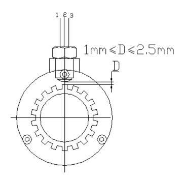
**Note:** Always screw in the sensor by hand when installation or adjustment.
