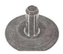
20. Check secondary sliding sheave wear.
