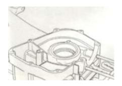
6. Clean gasket on crankcase contact face .
