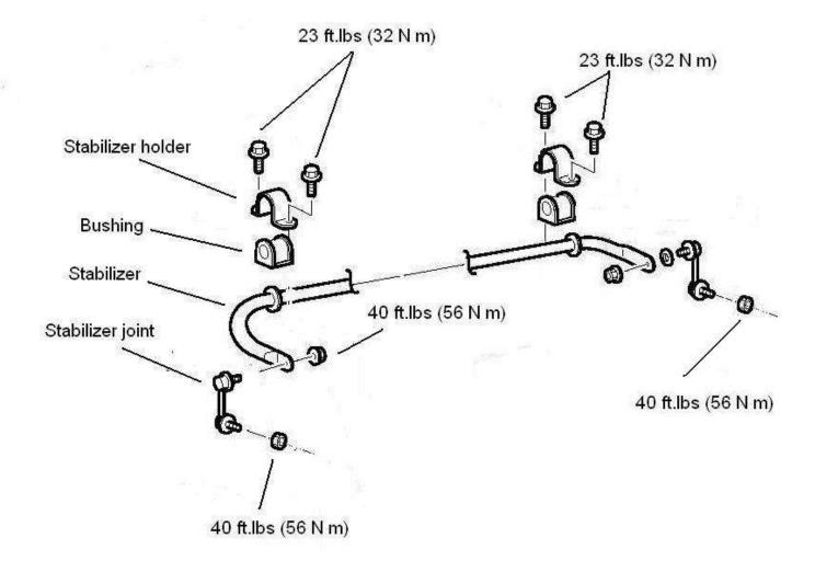
3. Remove the stabilizer bar nut from the lower A-arm, each side.
