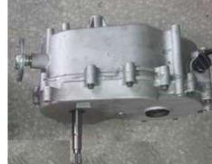
2. Remove transmission case fixing bolts.
