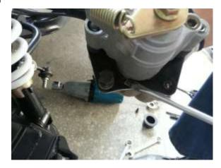
Measure the thickness of the caliper parking brake pads. Replace pads if worn beyond the service limit.
