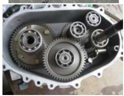
3. Knock the input shaft carefully with a soft face hammer to separate the transmission case from the left crankcase.
