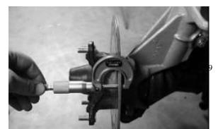
Measure the disc thickness at 8 different points around the pad contact surface using a 0-1" micrometer and a dial indicator. Replace disc if worn beyond service limit.
