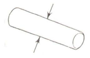
7. Measure piston pin outside diameter Limit: 14.96mm.
