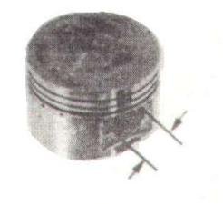
6. Measure piston pin bore diameter, Limit: 15.04mm.
