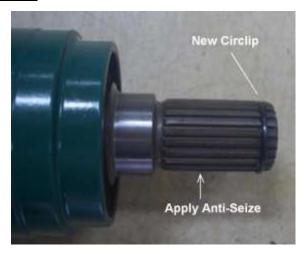
Reinstall the rear driveshaft into the rear gearcase. Be sure the circlip is securely fit into the rear gearcase. Use a rubber mallet to tap on the outboard end of the driveshaft if necessary.
