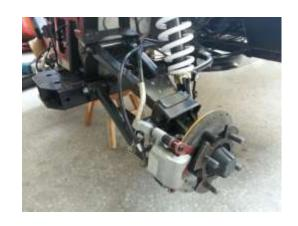
4. Remove the brake caliper. Suspend the brake caliper from the frame with a wire.
