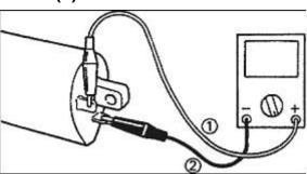
Tester (+) lead Spark plug lead Tester (— ) lead **Light Green Terminal**
