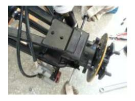
6. Remove the bolt that secures the shock and coil to the lower A-arm.
