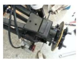
4. Remove the brake caliper. Suspend the brake caliper from the frame with a wire.
