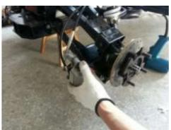
3. Remove the hub cap, cotter pin, spindle bolt, and washer.
