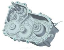
5. Remove the intermediate shaft assembly, the secondary axis assembly, and the output axis assembly in turn.
