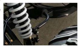
4. Remove the two bolts that secure the stabilizer bar to the main frame, each side.
