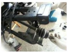
5. Loosen two bolts that secure the rear knuckle to the A-arm. Remove the rear knuckle assembly by sliding it off of the axle.
