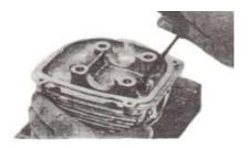
16. Measure valve guide inside diameter.
