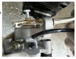
3. Inspect the brake lines and brake line connections for possible leaks or loose lines.
