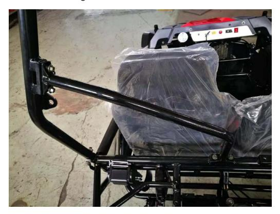
11、Assemble roll cage front: put front side of roll cage bar onto the connection rods on frame, fixing with bolt M8x55, R-washer and M8 nut. Then put back side onto the connection rods of roll cage rear, fixing with bolt M8x55, R-washer and M8 nut. The bolt is screwed on but not tightened.
