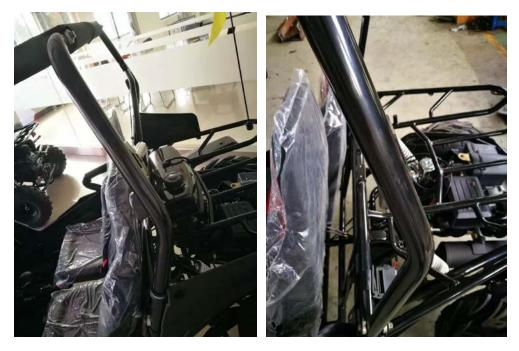
$10\,{\scriptstyle \scriptscriptstyle N}$  Assemble rear bar: put two sides of rear bar into the connection
