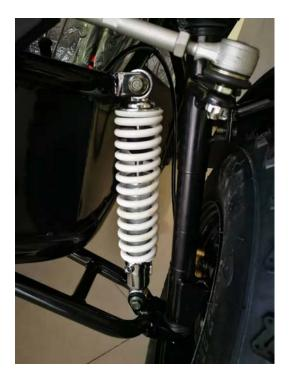
$7\,{}_{\sim}\,$  Assemble the front fender: take down the bolts M6\*16 on the strut,
