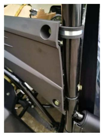
15.3 Use M6\*20 bolts and M6 flange nuts to connect and install the upper part of the rear plastic plate and the back part of the rear plastic plate. Tighten all bolts with a tightening torque of 11-16NM.
