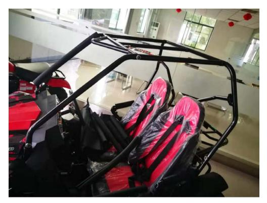
12、Assemble top cage: connect the top cage and roll cage front/ rear, fixing with bolt M8x55, R-washer and M8 nut. The bolt is screwed on but not tightened.
