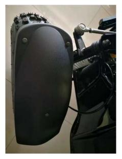
8、Assemble the front wheel: fit the front wheel onto the hub, screw the locking nut M10x1.25 tightly with 37-44NM. Use a crisscross sequence until they have reached their proper torque value. Then cover the hub cover.
