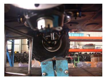
6. Assemble the front shocks: take down the bolt on the shocks, attach the shock on the front lower suspension arm and the shock mounting position of the frame, then fix the bolt with 37-44NM torque.
