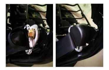
21、 Adjust the height of the steering wheel: after the driver sits on the seat and adjusts the seat to an appropriate position as required, loosen the bolts of the steering wheel adjusting installation bracket, then adjust the steering wheel to a comfortable height, and finally tighten the bolts.
