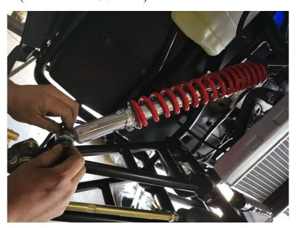
2.2 Assemble the rear shocks: Assemble the rear shocks to rear swing arm; use 37-44NM torque to fix the shocks attached the frame. (Note: 1NM = 0.74 lb ft)
