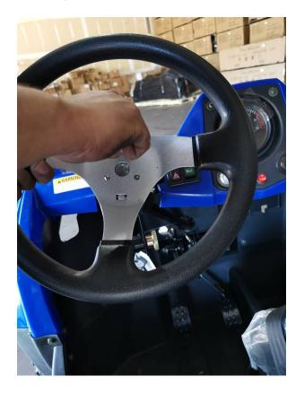
2.7 Adjust the steering wheel angle: loose the adjustment nut as shown in the picture, adjust the steering wheel to a comfortable height, tighten the nut
