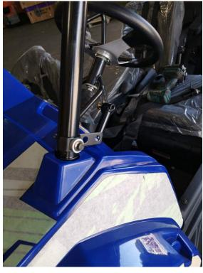
2.9 Install the rear roll cage bar: put the rear roll cage bar onto the mount posts of the frame, fix it using M8x55 bolt, R-washer and M8 nut.
