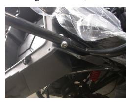
2.10 Joint the front and rear roll cage: joint the roll cages and connect them with M8x30 bolt and M8 nut. The recommended torque is 22-29NM
