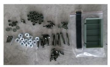
1.4.3 Bag 3: Steering wheel cover (1pc), cable for headlight (1pc), clamps for windshield (10pc), clamp cushion for windshield (4pc), plastic plug (2pc), self-locking nut M10X1.25 (2pc), bolt M5X25 (1pc), washer ∮ 5 (1pc), rear mirror mount and O-ring (1pc)
