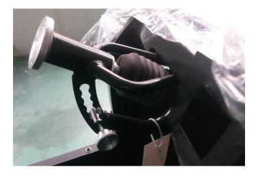
2.8 Install the front roll cage bar: put the front roll cage bar into the mount posts on the frame, put in the M8x60 bolt, R-washer, mirror bracket and tighten the M8 nut to fix.
