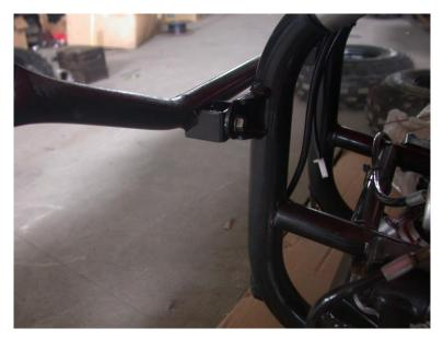
2.6 Set up the top headlights wire: open the right side of front hood cover as displayed in the picture, put the wire through the hole on the front hood cover where the front roll cage bar mount rod is, connect the plugs
