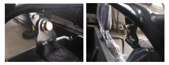
2.15 Install the seat back head rest (*No this step with new sport seat*!)
