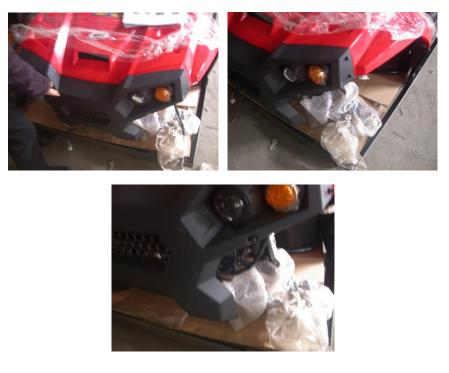
2.8 Plug the headlight and turn lights' wire: plug the wires with the connecting sockets; tighten the wires using zip ties.
