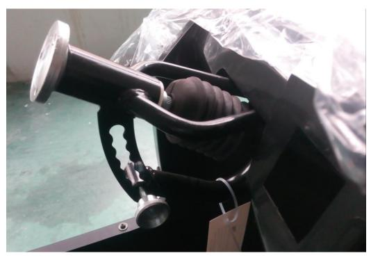
2.11 Install the front roll cage bar: put the front roll cage bar into the mount posts on the frame, put in the M8x60 bolt, R-washer, windshield bracket and tighten the M8 nut to fix.
