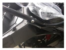
2.13 Joint the front and rear roll cage: joint the roll cages and connect them with M8x30 bolt and M8 nut. The recommended torque is 22-29NM
