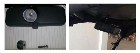
2.17 Install the canopy top: put the foam padding on the top roll cage, install the canopy top and tighten it.
