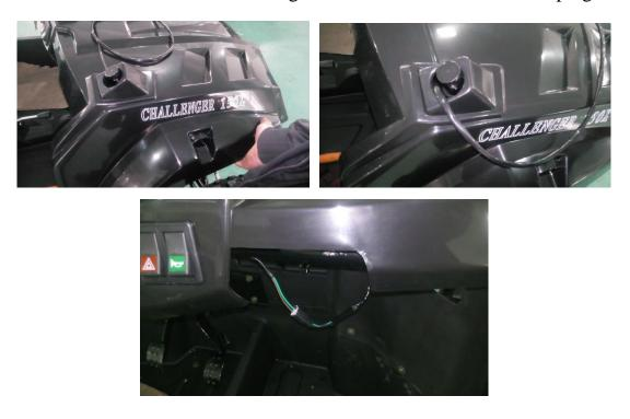
2.7 Install the front light cover: attach the front light cover on the frame and install it on the frame with M6X16 bolts and M6 nuts.
