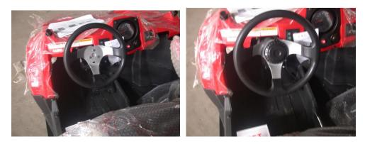
2.10 Adjust the steering wheel angle: loose the adjustment nut as shown in the picture, adjust the steering wheel to a comfortable height, tighten
