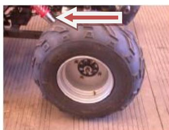
2.3 Assemble the front lower suspension arm (pic.18): lift the frame over the ground, take down the bolts and washers on the bulbs of strut, attach the lower suspension arm to the strut, put on the washer and castle nut in order, screw the nut with 55-62NM torque, fix the cotter pin 2.5X25 through the castle nut.
