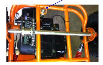
C. After the go-kart has been driven for a while, the <u>drive</u> chain on clutch will be loosen and should be readjusted. At first, <u>four bolts</u> fixing the engine on mount plate have to be loosen until the engine can be moved. Then, adjust the <u>chain adjusting</u> <u>bolt at the front side of engine</u> to tighten the chain to an appropriate tension. At last, after adjusting screw the four bolts tightly.
